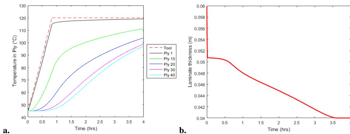
**Figure 2:** Results of the resin flow and heat transfer model; (a) significant thermal lag in the plies further from the tool surface, (b) laminate thickness reduction slows as the resin begins impregnating the tows. The heating rate was 1.5 C/min until the tool surface temperature reached 120°C and then it was held constant
