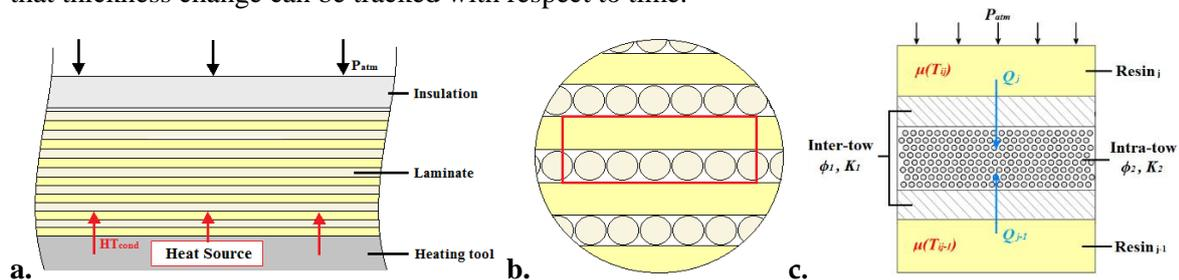
**Figure 1:** Physical representation of the model; (a) a thick laminate (40 mm) has heat applied from the bottom surface and is insulated on the top surface, (b) the laminate is made up of ‘semi-preg’ plies, which can be viewed as unit cells, (c) the unit cell in the model can account for flow from both its own resin layer and the resin layer below.
